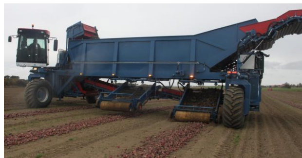
Fig. 2. Prototype wide span tractor configured for onion harvest.
