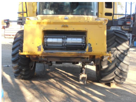
NH CR940 combine. Left with a 520 mm CTF tyre. Right a 900 mm tyre for other fields.
